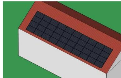
Figure 3 PV modules packed too closely for safe access and efficient maintenance.
