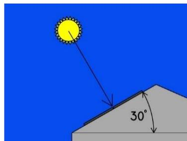
Figure 1 Near-optimal tilt for year-round generation in New Zealand.
