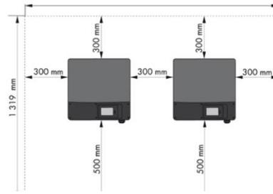
Figure 5 Example of spacing recommended for SMA wall mounted inverters. From <https://www.sma-sunny.com><sup>31</sup>
