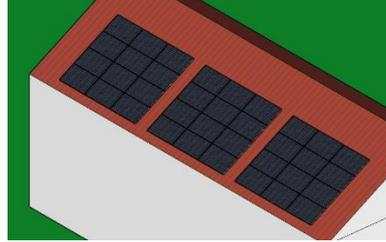
*Figure 4 Larger array split to allow access by maintenance personnel.*
